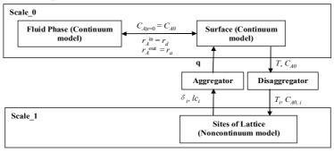
Figure 8: Structure of the heterogeneous reactor model.
